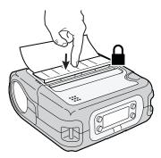
**6** Pull on the liner to tighten it and ensure a good self strip.
